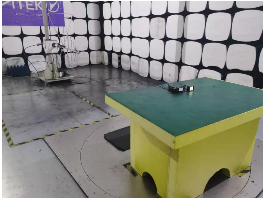
Spurious Emission Test Setup (Below 1GHz)
