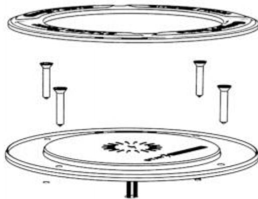
Step 3: Place the Silicon non-slip ring onto the top of the Charging Cap using the adhesive tape.
