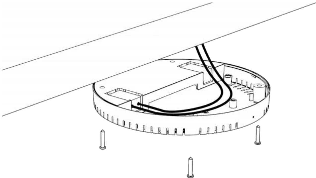
Step 2: Securely mount the Wireless Charging Module to the bottom of the surface using four (4) screws and/or the high-strength double-sided tape if screwing into the surface is not feasible.
