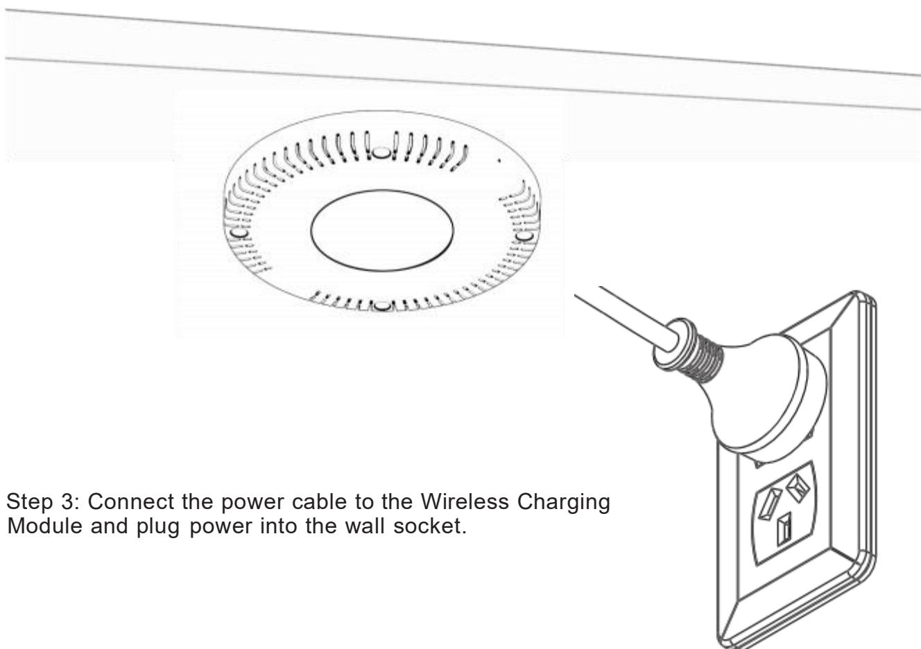
Step 3: Connect the power cable to the Wireless Charging Module and plug power into the wall socket.
