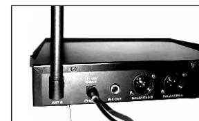
4. Connect receiver to mixer or amplifier. Make sure audio levels on the mixer are muted or off. For PA System, use the 1/4" AF output (line level unbalanced, 4b). For all other applications use the XLR output (mic level 4a)
