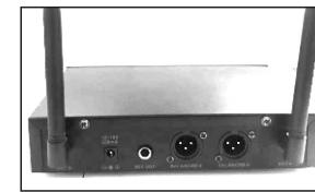
3. Connect power supply. Plug in the DC power supply ( 110-240V, DC 13.5 V 350mA )
