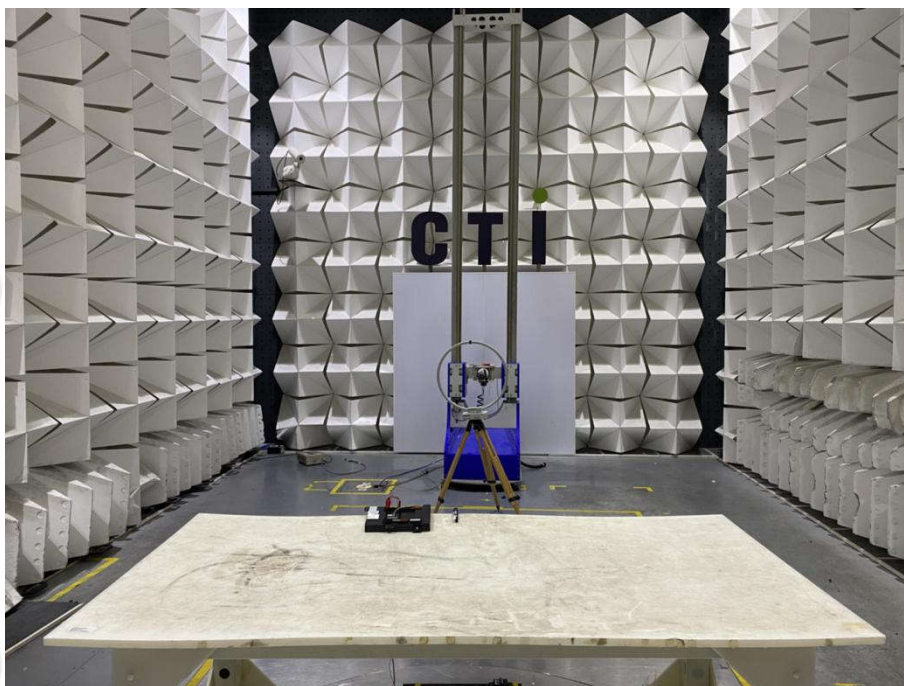
Radiated Spurious Emissions Test Setup (9kHz~30MHz)
