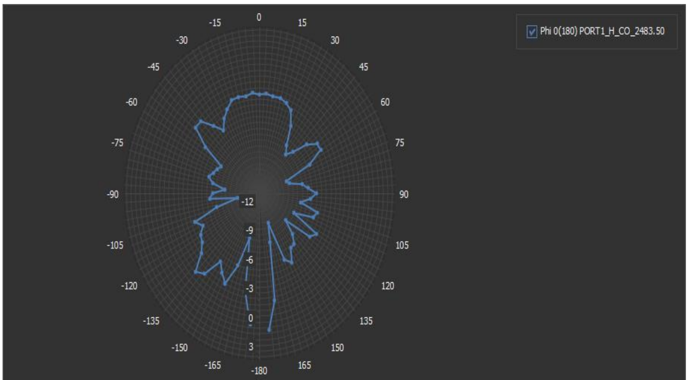
Figure 6: Sample 1 (2D radiation direction diagram, 2483.50MHz, Phi=0 ° /180 ° )
