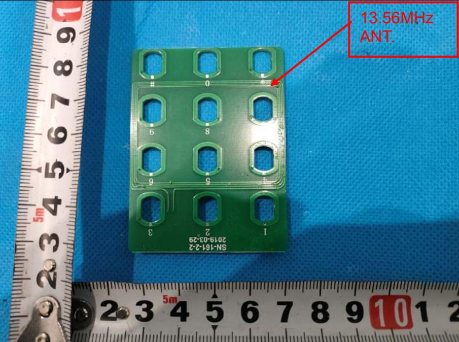
A photograph of a green printed circuit board (PCB) with a central rectangular aperture. The PCB is placed next to a metric tape measure. A red box with the text '13.56MHz ANT.' is overlaid on the image, pointing to the central aperture. The PCB has some surface text and numbers: '2019-2', 'SN-161-22', '3', '1', '6', '8', '6', '6', '0', '#', '8', '6', '6', '3', '1', '2', '9', '1', '2', '3', '4', '5', '6', '7', '8', '9', '10', '1', '2'. The tape measure shows markings from 1 to 10 centimeters.
