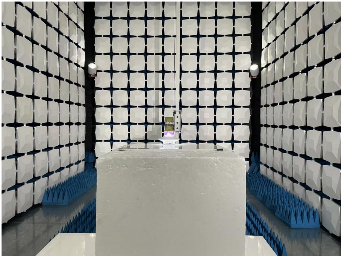
Above 1GHz for radiated emission test setup
