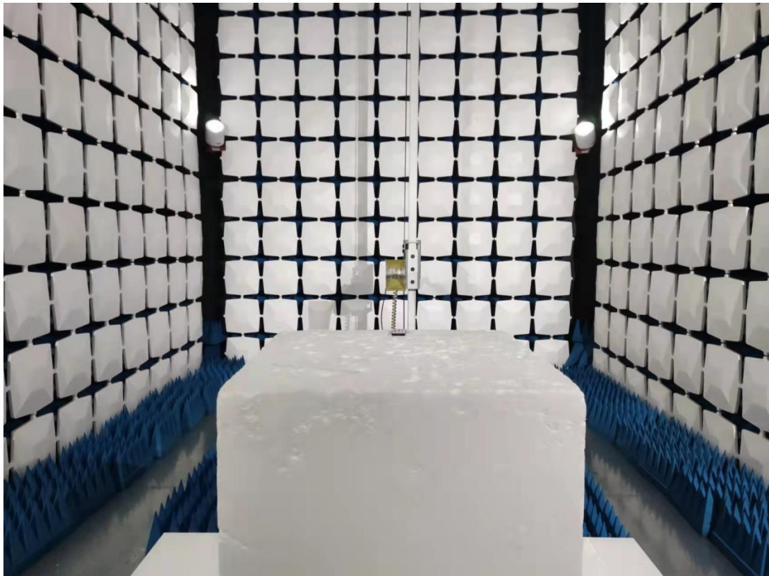
Above 1GHz for radiated emission test setup
