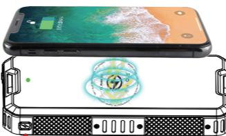
**IMPORTANT:** Press the power button to activate the battery after placing your phone on the power bank.
