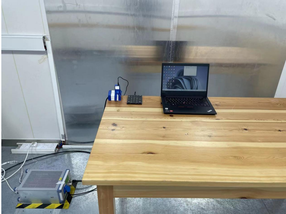
Conducted emission test setup
