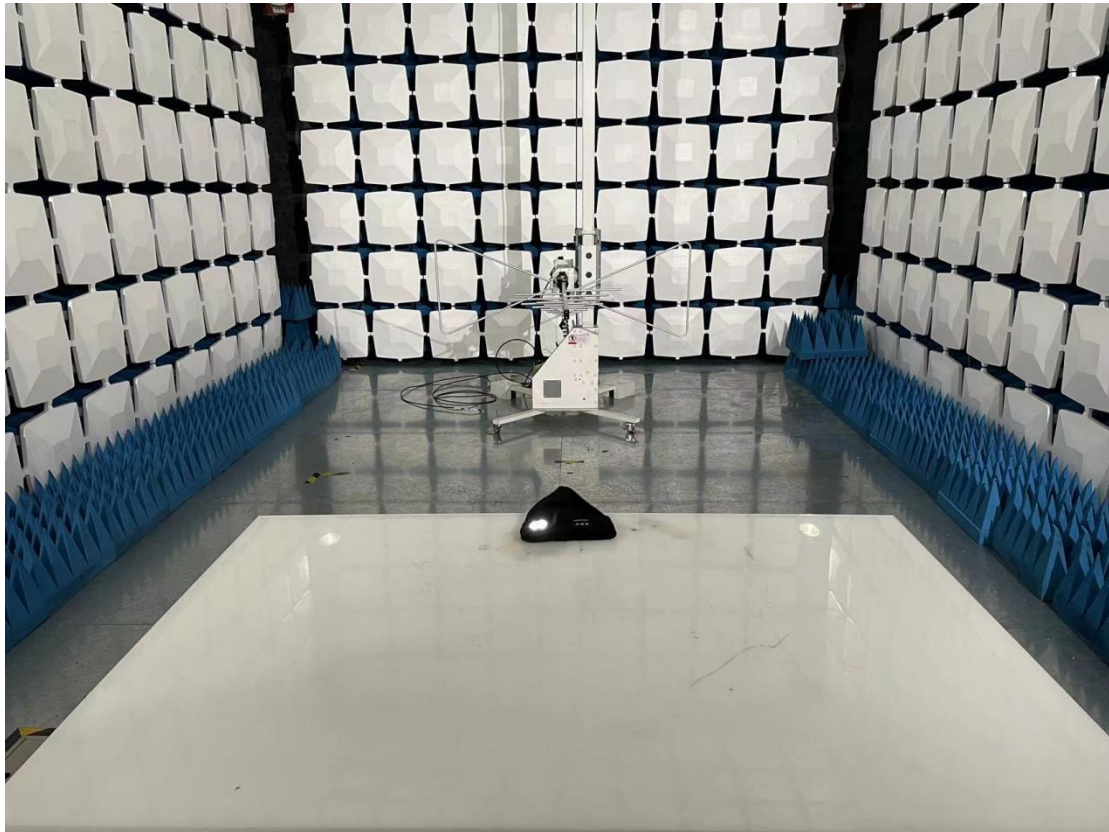
Above 1GHz for radiated emission test setup
