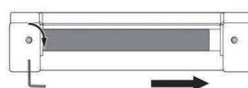
If deviating turns to left, then turn the left screw in clockwise direction, turn the right screw in counterclockwise direction.
