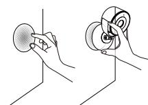
Remove the plastic cover from the adhesive tape, place the camera on the ideal spot on the wall or ceiling, wait a few seconds for it to set, and then conveniently adjust the angle and orientation by hand, considering the cable's maximum range of 9 ft.
