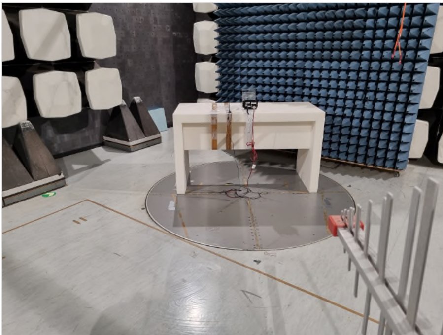
Photograph 12: EUT test setup in the semi anechoic chamber without floor absorber for E-Field measurement, overview_EUT elevation 90°
