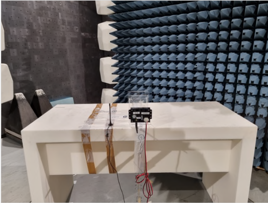
Photograph 11: EUT test setup in the semi anechoic chamber without floor absorber for E-Field measurement, close up view_EUT elevation 90°
