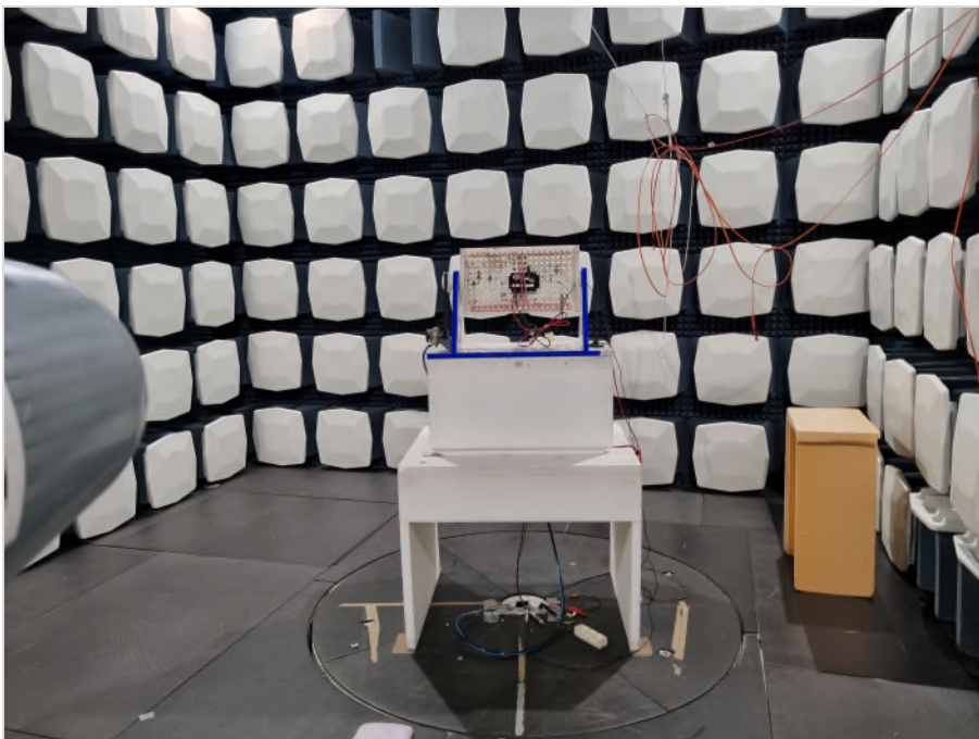
Photograph 4: EUT test setup in the fully anechoic chamber, overview_EUT elevation 90°
