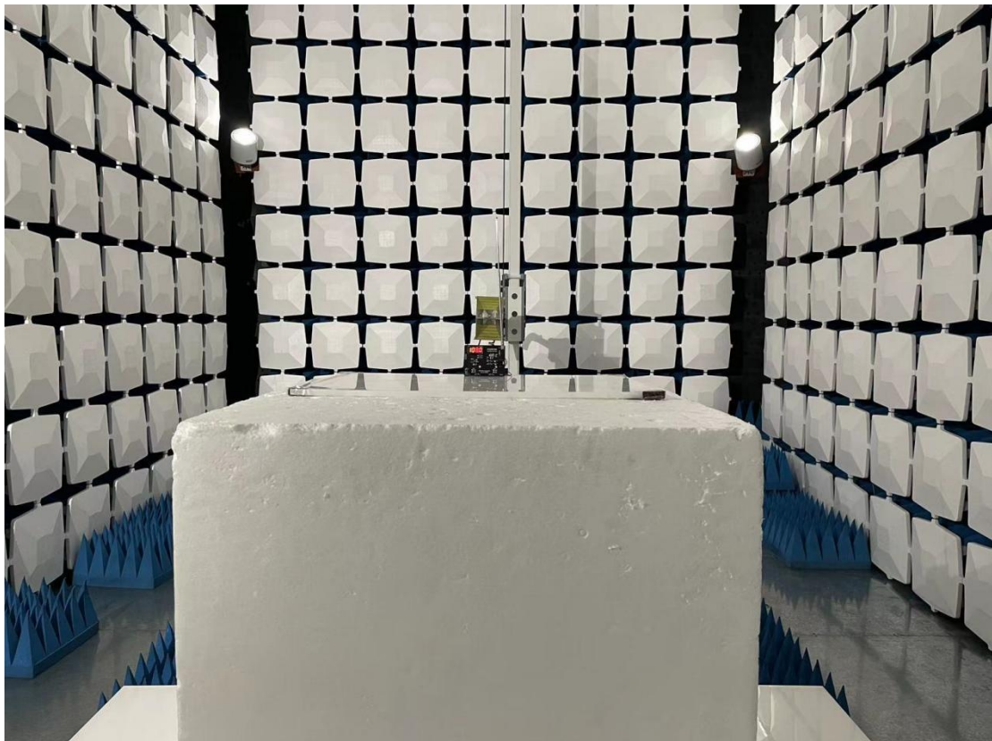
Above 1GHz for radiated emission test setup
