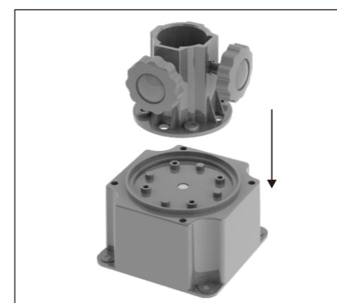
A: Place Main Pole Column onto Motor-Fixed Bolster.
