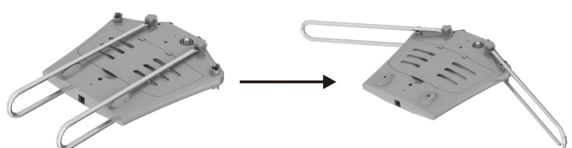
A: Rotate the VHF receiving vibrator on the main body into the card slots on both sides.
