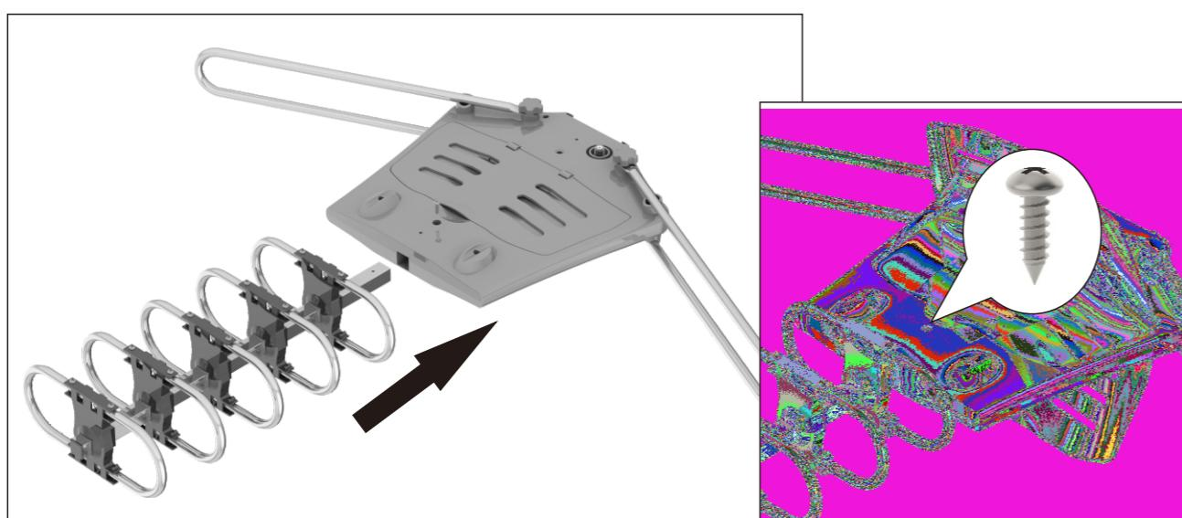
C: Insert the new assembly into the Main Unit as shown.
