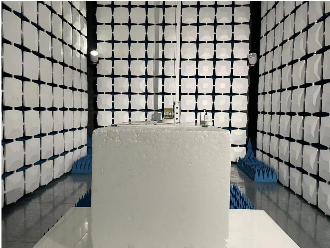
Above 1GHz for radiated emission test setup
