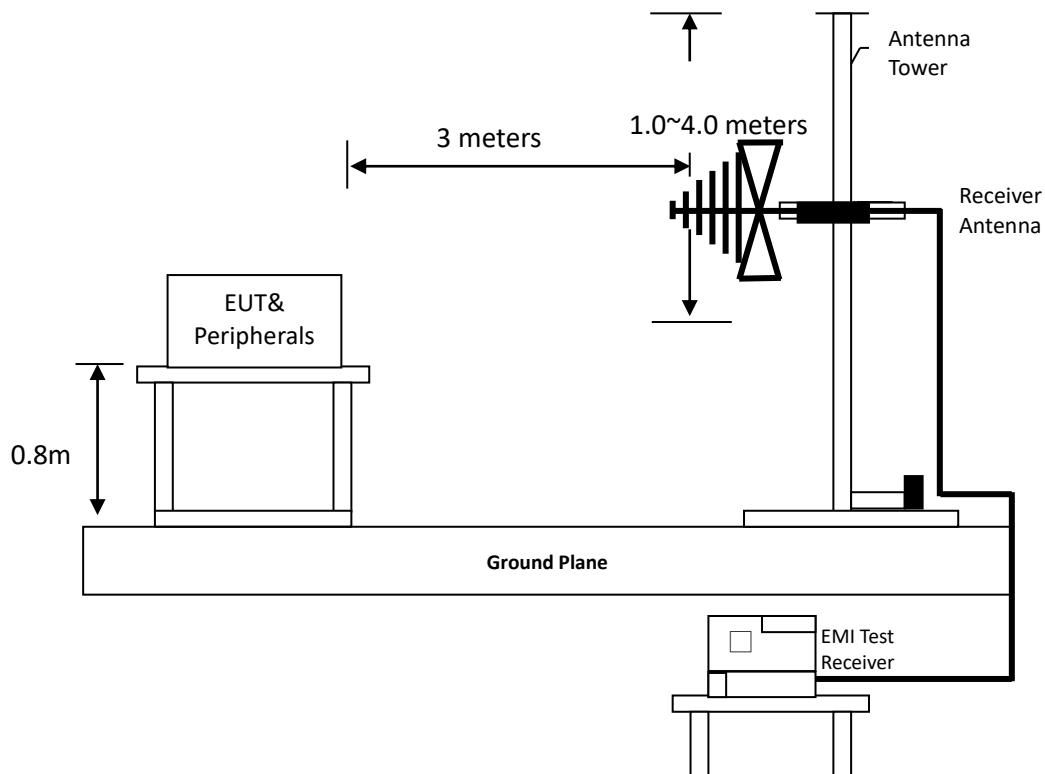
Radiated emissions were investigated cover the frequency range from 30MHz to 1000MHz using a receiver RBW of 120kHz record QP reading, and the frequency over 1GHz using a spectrum analyzer RBW of 1MHz and 10Hz VBW record Average reading. (15.209 paragraph), the Peak reading (1 MHz RBW/ 3 MHz VBW) recorded also on the report.
