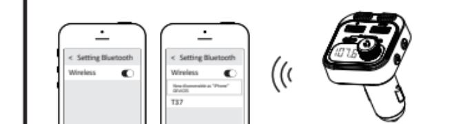
4. Turn on your car's FM radio and find an empty (synthetic) station. Then, adjust the frequency on T37 to match the frequency of your car radio.
