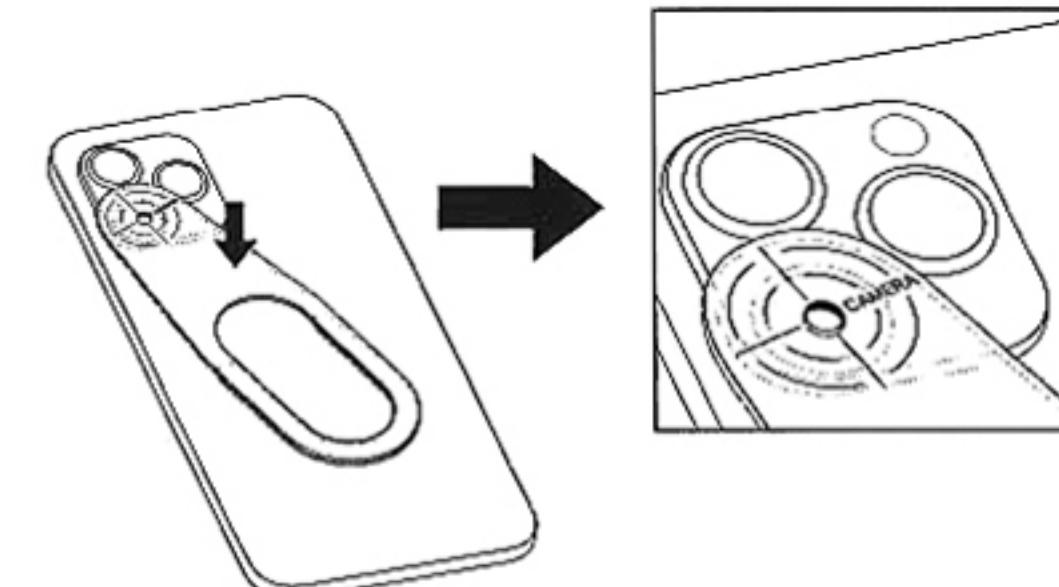
Make sure that the center of the scribing ruler is consistent with the center of the lens. To prevent the end of the scribing ruler from detaching from the phone, stick the scribing ruler after finding the proper position.
