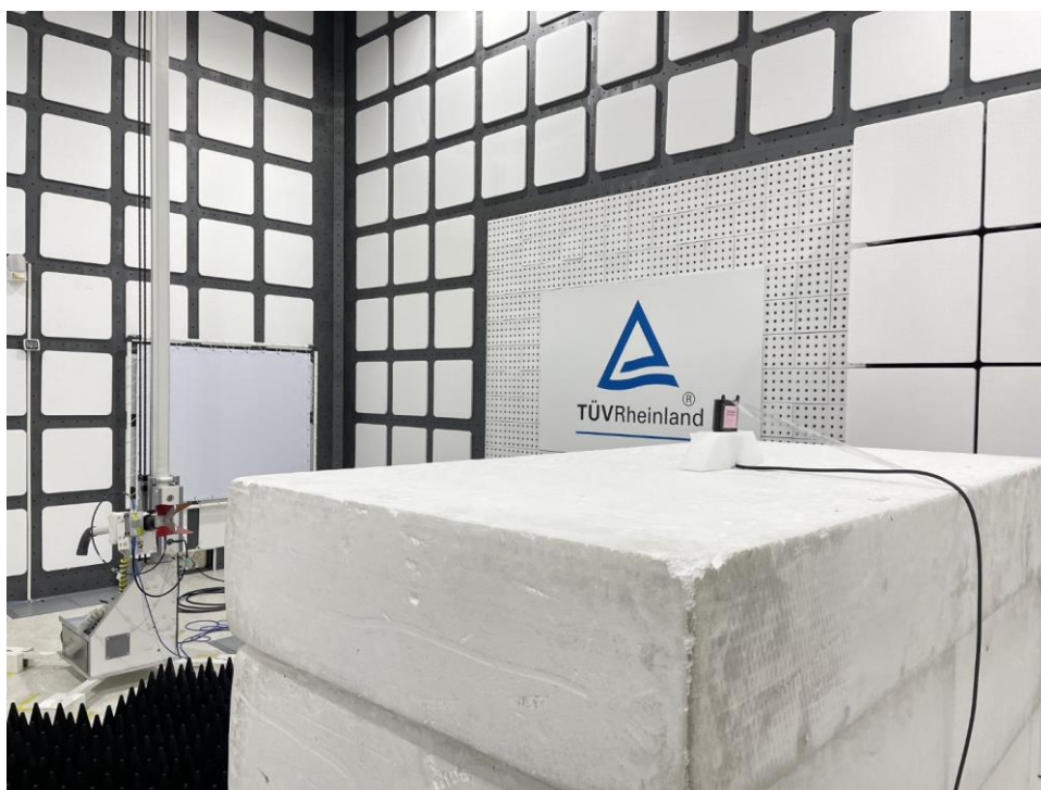
Photograph 4: Set-up photo for Radiated Spurious Emission, 18GHz to 40GHz
