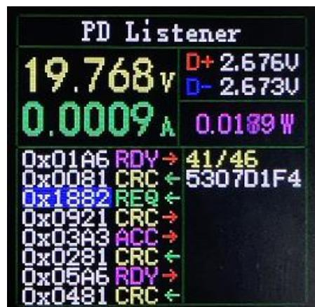
Click the middle button to switch to the "View Detailed Communication Process" page, as shown in the figure above.
