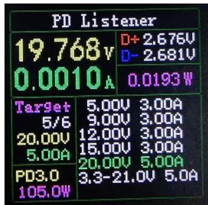
In the figure above, the charger is a 105W PD charging head. The current PD consumer selects the 5th gear and triggers the target voltage of 20V, the maximum current is 5A.
