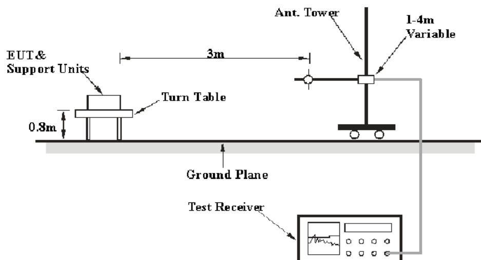
The radiated emissions were performed in the 3 meters distance, using the setup accordance with the ANSI C63.10-2013. The specification used was the FCC 15.209 and FCC Part 15.235(a) & 15.235 (b) limits.
