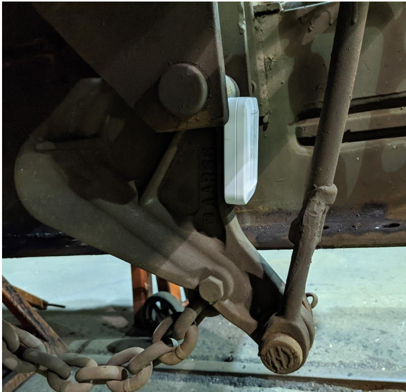
FIGURE 10 THE NORMAL MOUNTING LOCATION FOR THE HANDBRAKE SENSOR IS LOCATED ON THE SECTION OF ROTATING LEAF ASSEMBLY.
