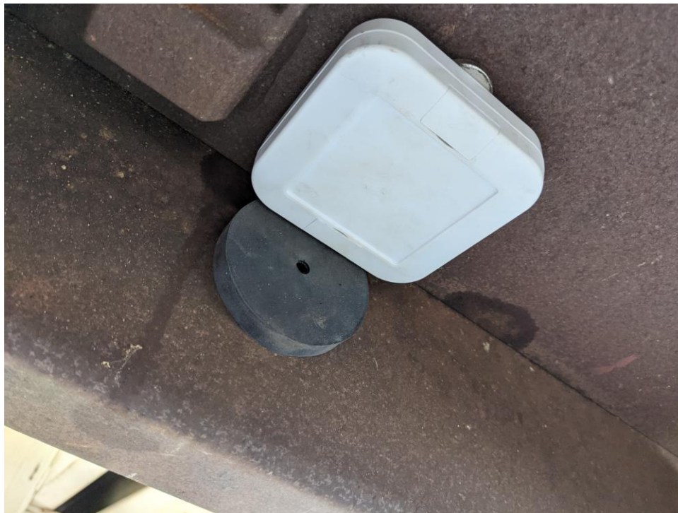
FIGURE 12 MOUNTING LOCATION FOR HOPPER CARS TO DETECT IF THE GATE IS OPEN. (CLOSED POSITION SHOWN)
