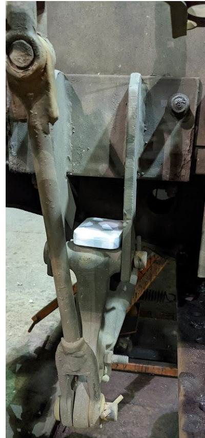
FIGURE 10 THE NORMAL MOUNTING LOCATION FOR THE HANDBRAKE SENSOR IS LOCATED ON THE SECTION OF ROTATING LEAF ASSEMBLY.
