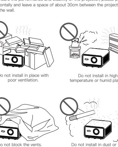
Do not install in place with poor ventilation.
