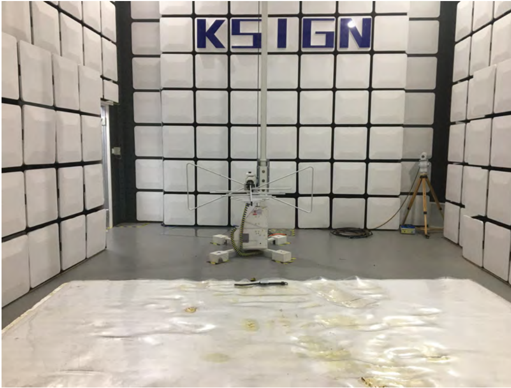
Radiated Measurement (Above 1GHz)
