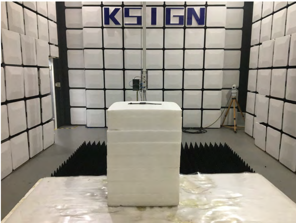
Radiated Measurement (Above 1GHz)
