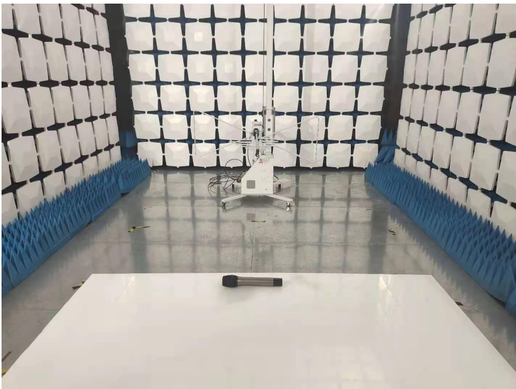
Below 1GHz for radiated emission test setup
