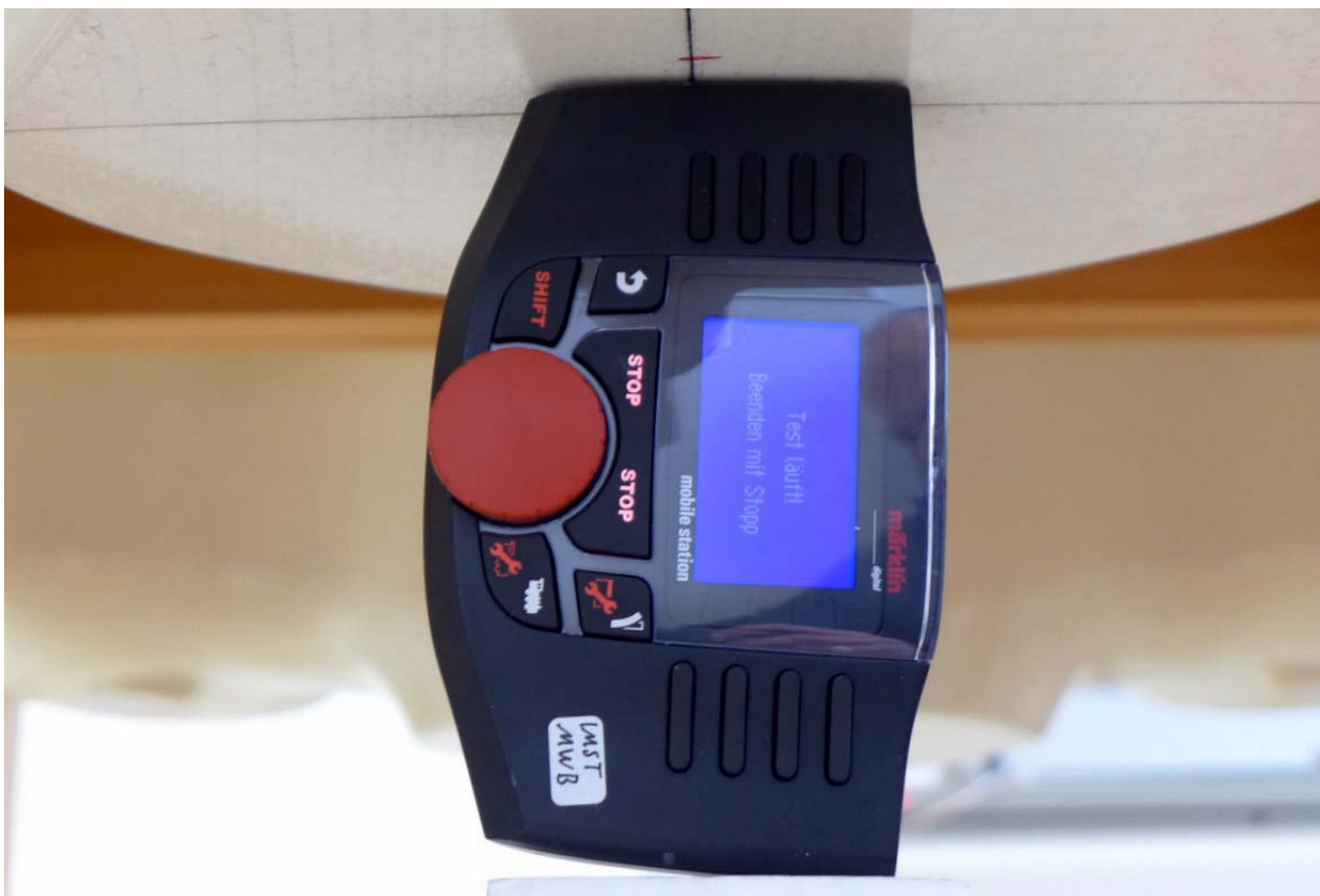
Pic. 7: Test position left side of DUT towards the phantom, 0 mm gap.
