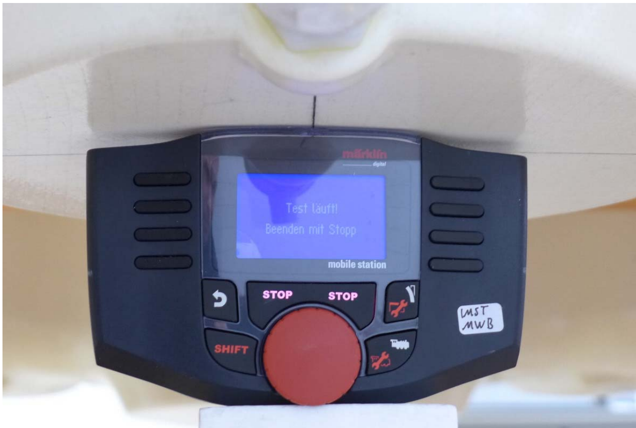
Pic. 9: Test position top side (1) of DUT towards the phantom, 0 mm gap.
