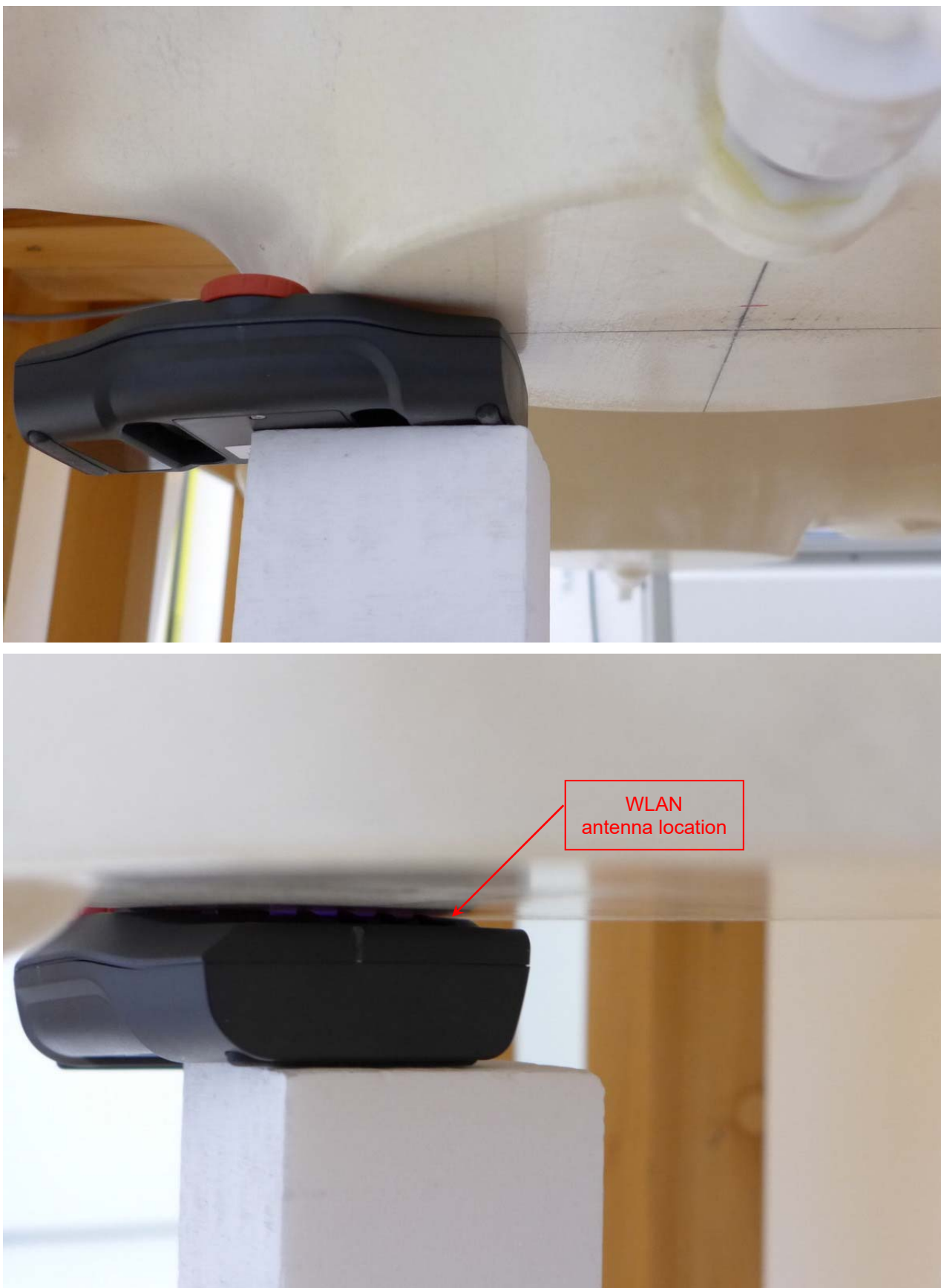
Pic. 5: Test position right part of the front side (2) of DUT towards the phantom, 0 mm gap.
