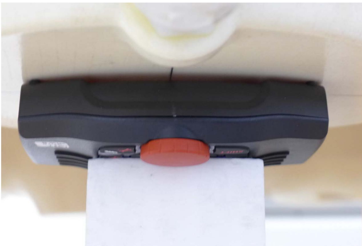
Pic. 6: Test position rear side of DUT towards the phantom, 0 mm gap.
