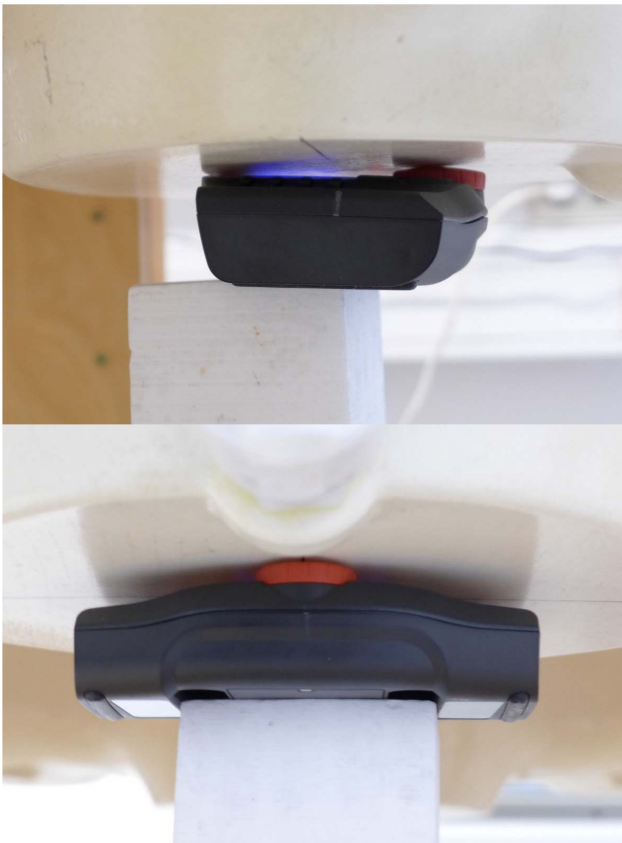
Pic. 4: Test position front side (1) of DUT towards the phantom, 0 mm gap.
