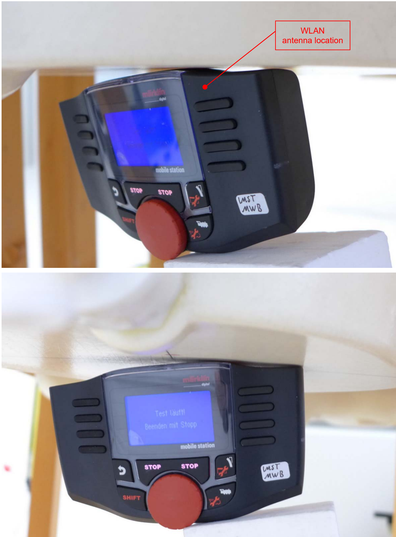
Pic. 10: Test position top side (2) of DUT towards the phantom, 0 mm gap.
