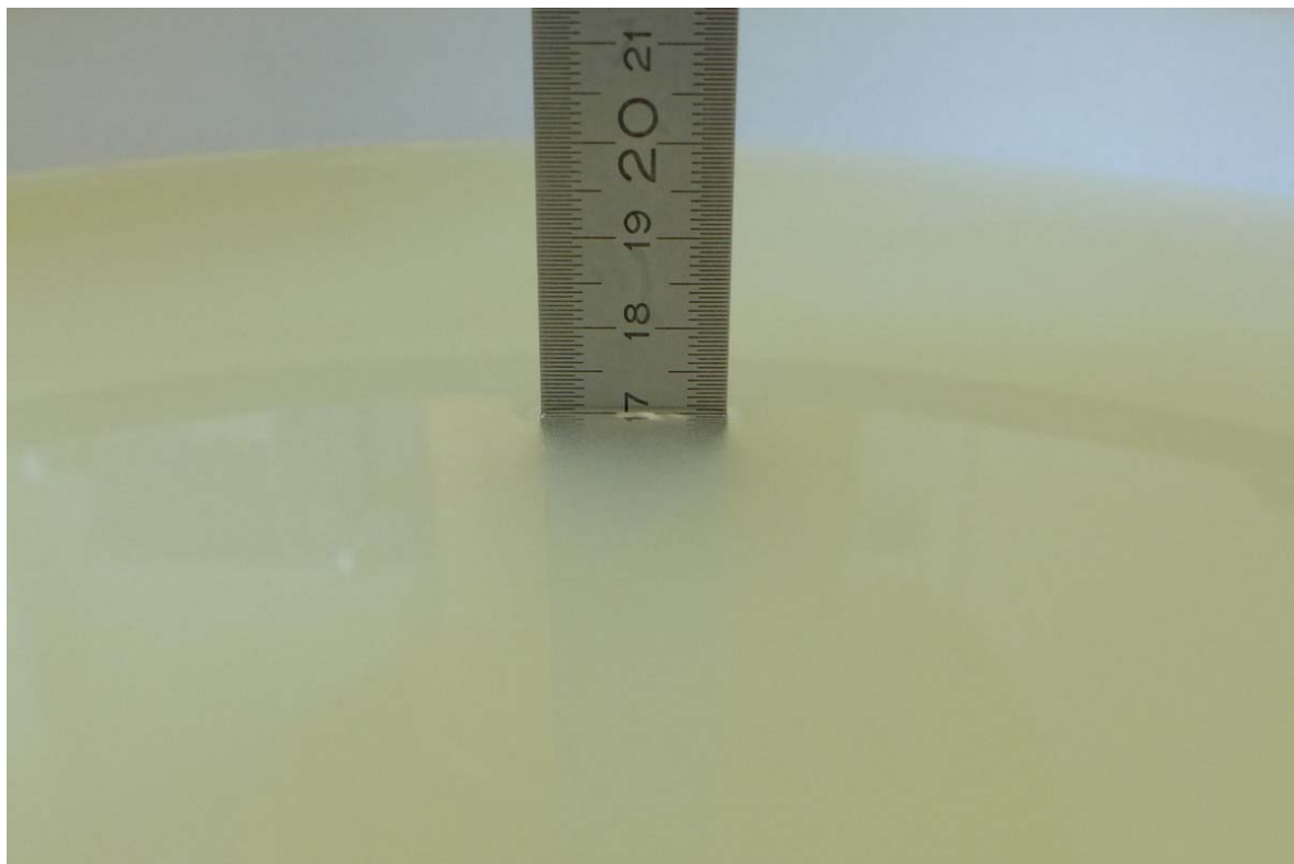
Pic. 11: Liquid depth for 2.4 GHz measurements.
