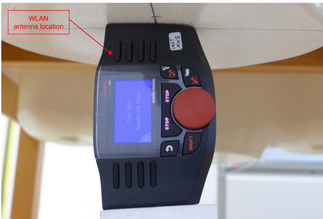
Pic. 8: Test position right side of DUT towards the phantom, 0 mm gap.
