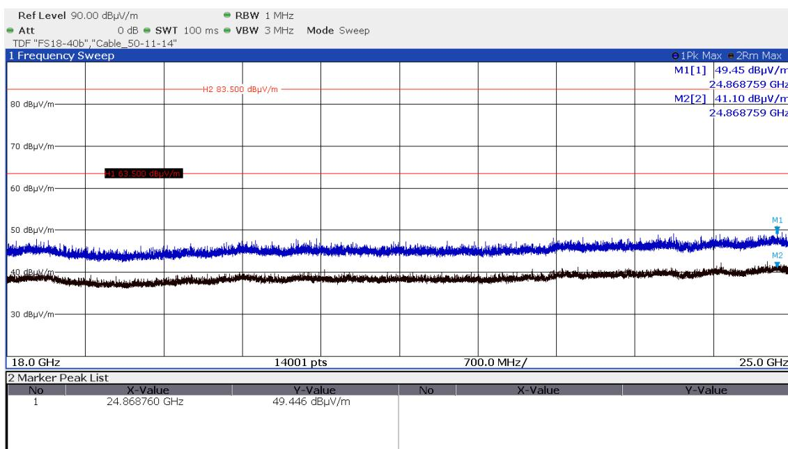
Note: The measurement distance for 18 - 25 GHz frequency range was changed to 1 m therefore the limit lines are adjusted and increased by 9.5 dB.
