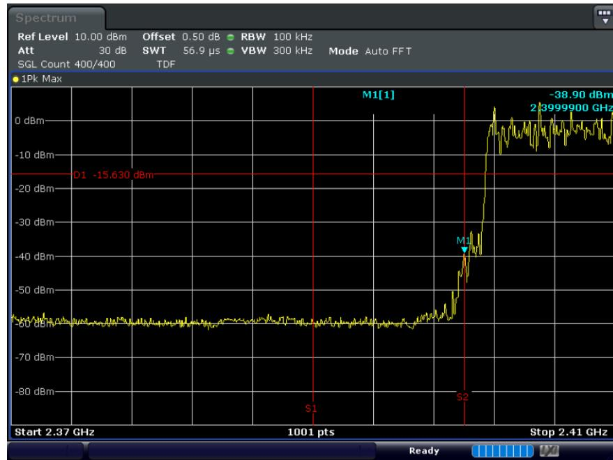
**A.3. Lowest Ch. (2 402 MHz)\_Spurious emissions**
