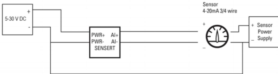
The sensor's 4-20 mA 3/4 wire supply need to share the same negative net with SENSERT power negative net.
