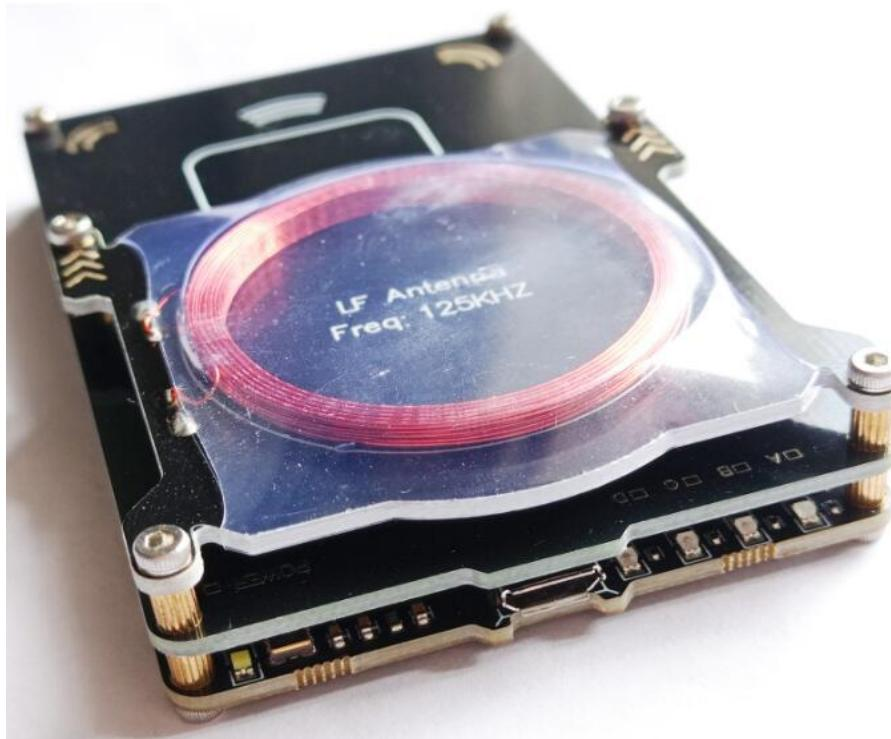
**Tip:** The low-frequency antenna can also be installed in four symmetrical positions on the top, bottom, left, and right, and you can choose according to your preferences. In the recommended way, the two antennas have the least influence on each other.
