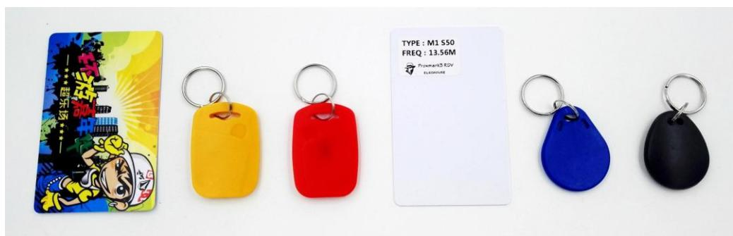
ID card: read the card ID number → replace the T5577 card → write the ID number into the card → complete
