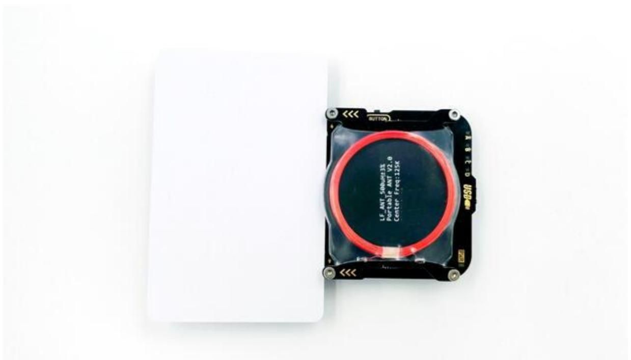
Place the card as shown in the picture above. Normally, there is no problem. In addition, please keep away from metal objects and metal tabletops. Individual keychains or small cards with poor signals can easily interrupt the reading and writing. At this time, you can read the card as shown in the figure below and put the low-frequency antenna under the high-frequency antenna to solve the problem.
