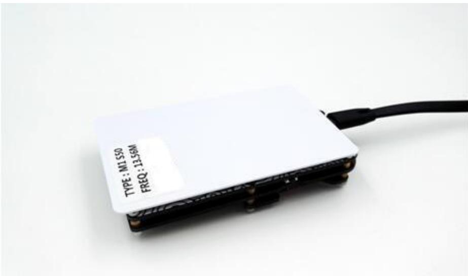
**The IC card is recommended to be placed on the back of the device and aligned with the device, which is the most stable.**
