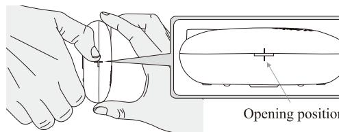
② Align the positive and negative directions respectively, and install 2 AAA batteries.
