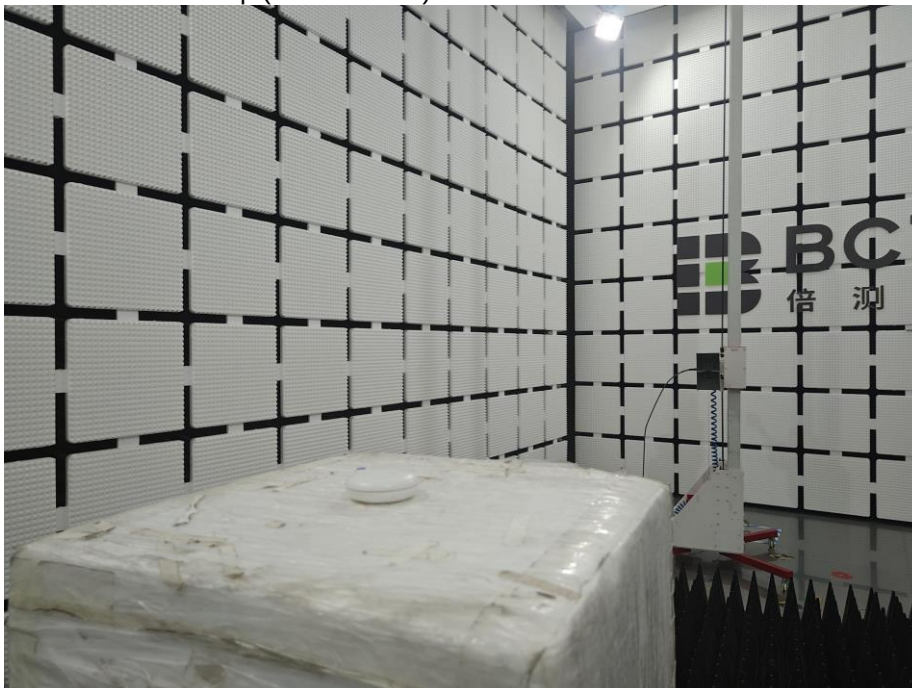
Spurious Emission Test Setup (Above 1GHz)
