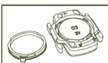
4. Align the battery cover to the unlocking position, turn it in the direction of tight locking, and tighten.
