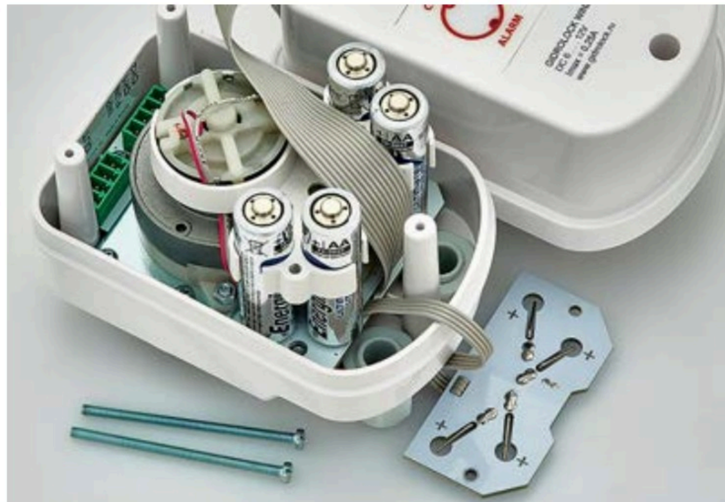
Photo 31. Contact plate is removed, batteries can be replaced
