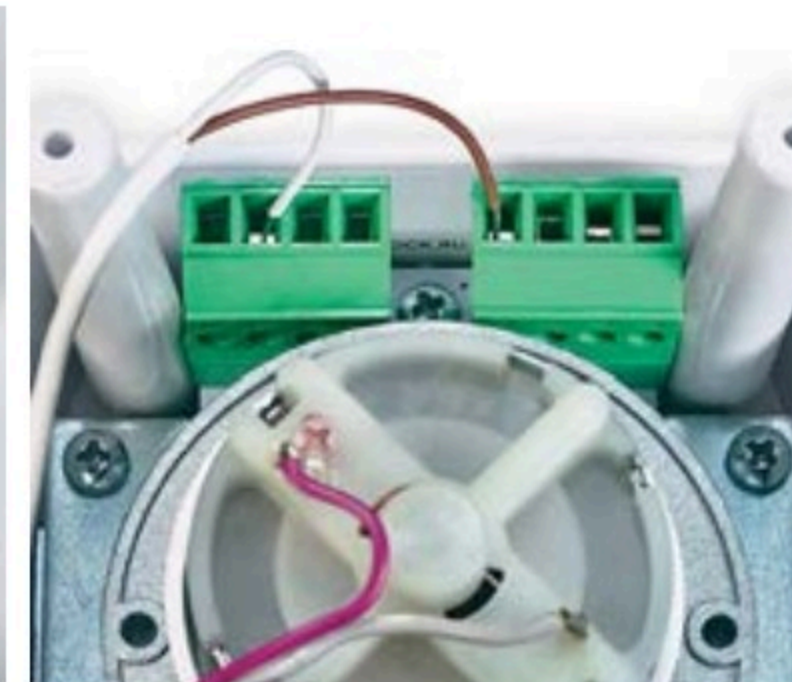
Photo 11. Connecting the sensor to the electric actuator
