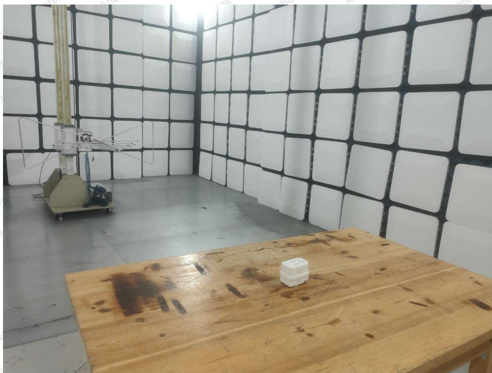
Photo of Radiation Emission Test
