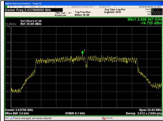
IEEE 802.11g Channel 6 20MHz_Antenna 0
