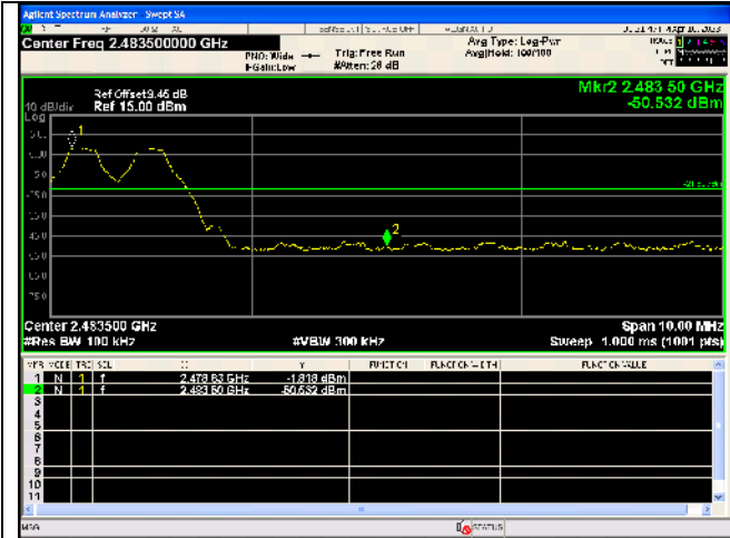
Out Of Band Emission(Right) GFSK_DH5_Channel Hopping
