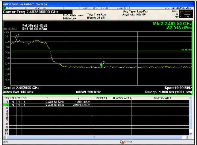
Out Of Band Emission(Right) 8DPSK_3-DH5_Channel Hopping
