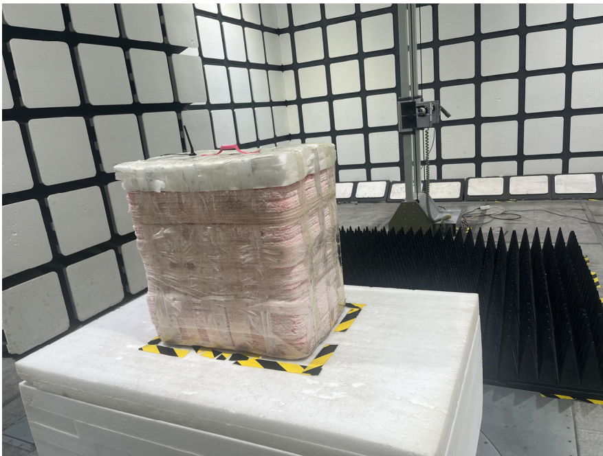
Radiated Emissions View (1-18 GHz)
