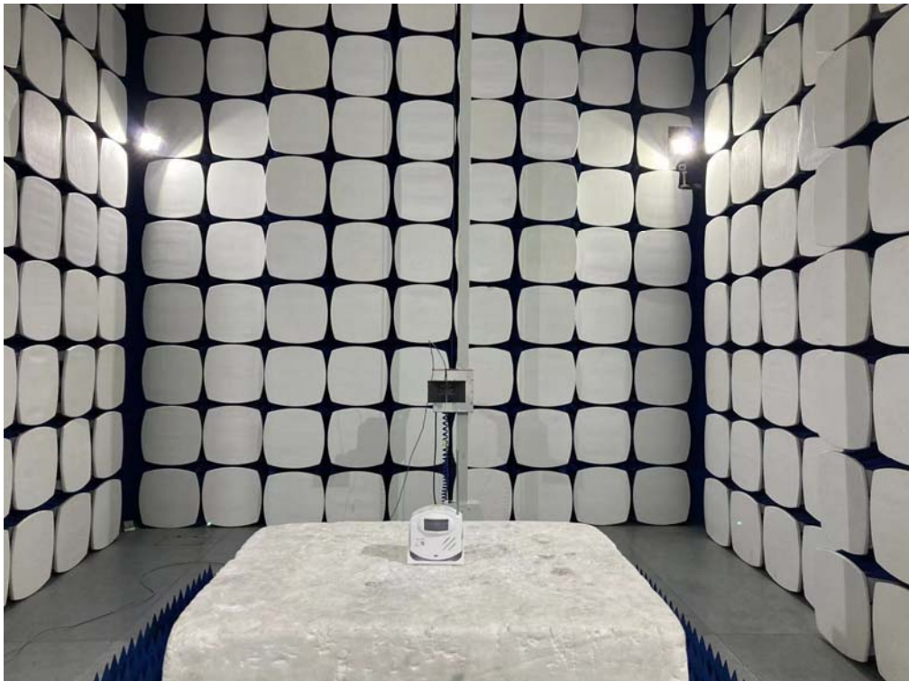
Radiated Setup photo (Above 1G)
