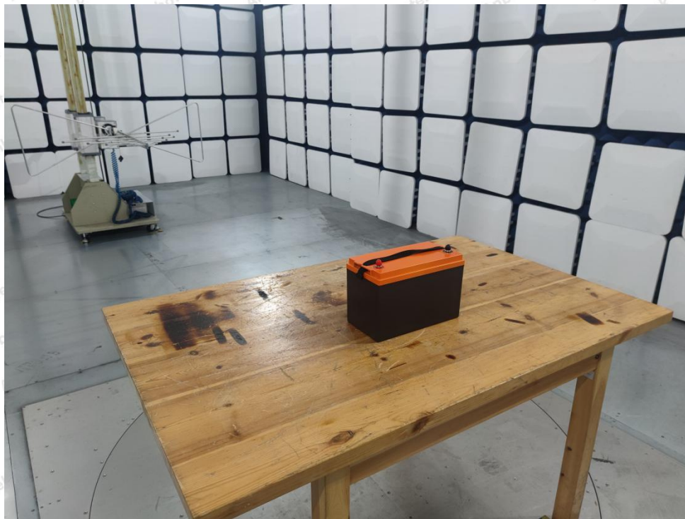
Photo of Radiation Emission Test
