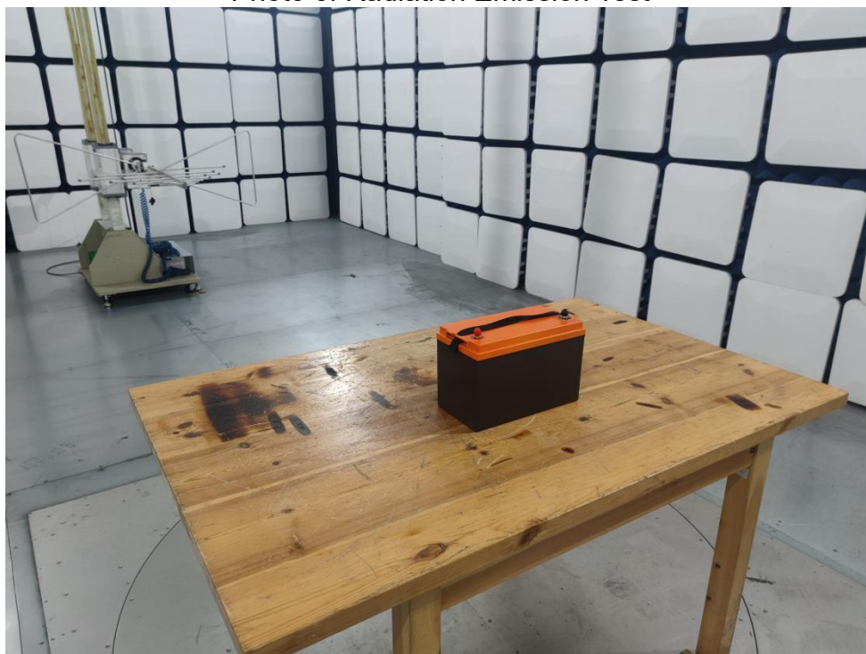
Photo of Radiation Emission Test
