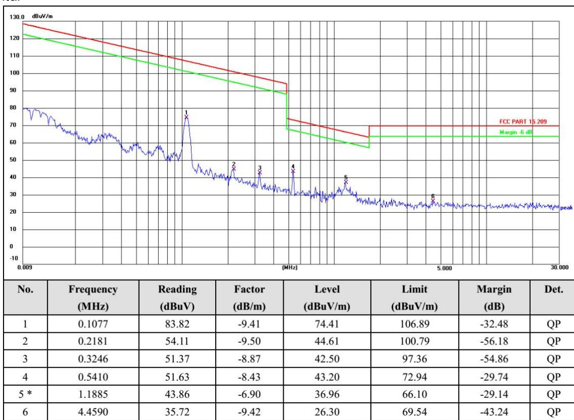
Remark: 1). Measured at antenna position 0 degree and 90 degree, recorded worst case at 0 degree.
