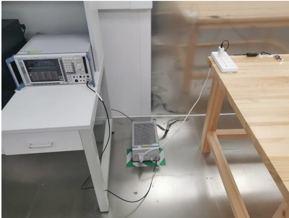
Test Setup Photo of Line Conducted Emissions Measurement
