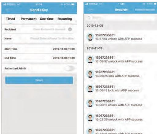
After adding the lock successfully, the user has the highest authority of the lock, which is the administrator of the lock. The user can send the bluetooth key to others with setting the time limit, and has the right to select the limited time, permanent or one-time Bluetooth key. The key is sent to recipient's mobile phone or email and the recipient will get the key and authority of the lock in the TTLock App.
