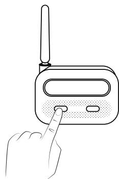
3. Press and hold the "P" button on the GPS collar receiver for 3 seconds to turn it on.
