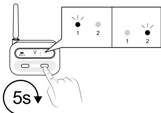
5. Press the M button on the GPS collar receiver, and the pairing icon will be displayed.
