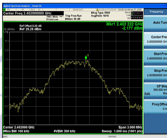
GFSK: Band Edge, Left Side
