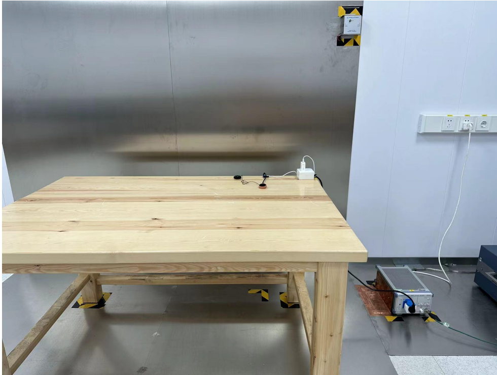
Radiated Emission Test View (Below 1G)
