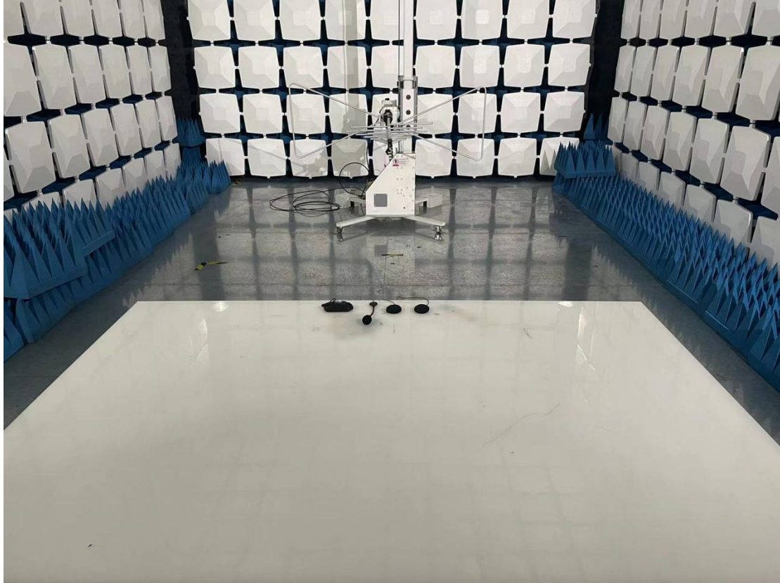
Above 1GHz for radiated emission test setup
